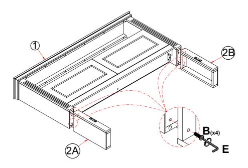
STEP 2: Attach crossbar (9) onto the left leg frame (2A) and right leg frame (2B) using the bolts (B), tighten it up by using an allen key (E). Later, attach adhesive felt pad (F) onto the legs.
