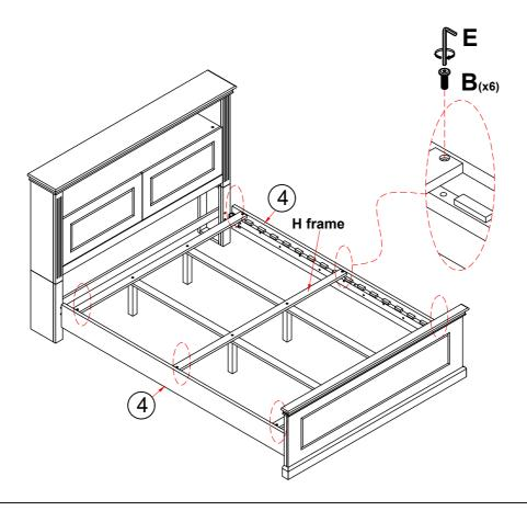
STEP 6: Once the bed is positioned and the support legs are adjusted to touch the floor, the slats can then be laid down and secured before placing the mattress on top.
